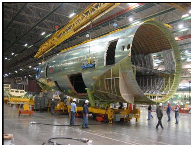
Figure 2: Mobile “crawlers” contain the PLC’s that manage the safe and reliable assembly of aircraft
